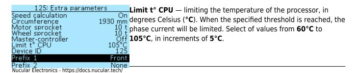
**Device ID** — setting the Controller number in the CAN network. This number is displayed in the menu section **Settings** > **Devices** in front of each device that is connected to the network using the **LEVCAN** protocol. If, by default, your device number is **0**, we recommend changing it to another number for the correct firmware update.
