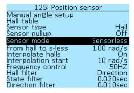
**Hall filter** — enable or disable the filter in the direction of rotation, select the **Direction** and **OFF** values.
