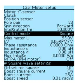
**Pole pair** — the number of pole pairs of the stator winding of the electric motor determines the speed at which the motor shaft will rotate. This parameter is used to calculate RPM and speed. For a
