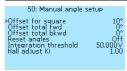
**Offset for square** — additional shift for square wave mode, in degrees (°). Select of values from -30° to 30°, in increments of 1°.
