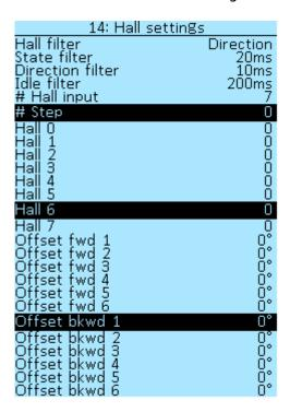
**Hall filter** — enable or disable the filter in the direction of rotation, select the **Direction** and **OFF** values.
