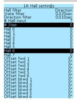
**Hall filter** — enable or disable the filter in the direction of rotation, select the **Direction** and **OFF** values.
