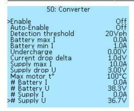
**Enable** — turn on the converter mode and start charging. Select of values **On** and **Off**.
