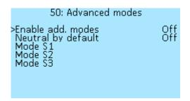
To activate the control modes, select **Controller > Advanced modes > Enable add. modes** and to set **On**.
