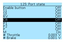
In the section **Controller** > **I/O configuration** > **Port state**, you can check input activation when contact shorted to GND. When a signal is applied, the value will change from **Off** to **On**. Below in the menu items **# Throttle** and **# Brake** you can see the voltage on the throttle and brake levers, respectively.
