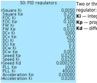
Two or three coefficients are used for the settings of each regulator:
