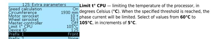
**Device ID** — setting the Controller number in the CAN network. This number is displayed in the menu section **Settings** > **Devices** in front of each device that is connected to the network using the **LEVCAN** protocol. If, by default, your device number is **0**, we recommend changing it to another number for the correct firmware update.
