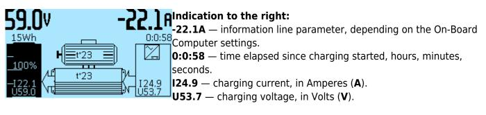
The indication in the middle is the temperature of the motor and the controller, respectively, in degrees Celsius (°C).
