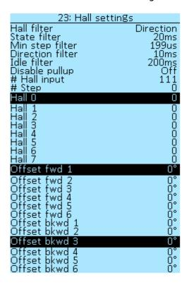
**Hall filter** — enable or disable the filter in the direction of rotation, select the **Direction** and **OFF** values.
