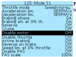
Throttle mode — selection of the operating mode of the throttle Speed+torqu. lever, read more in the section Throttle control mode setup.
