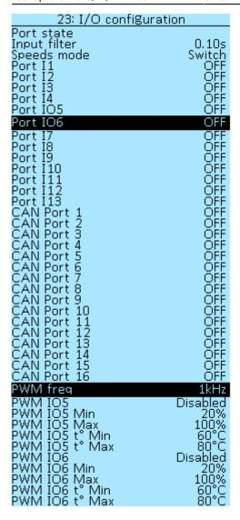
Available functions for the Controller ports I1, I2, I3, I4, IO5, IO6, I7, I8-I13 and CAN ports CAN port
