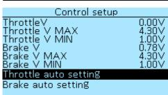
ThrottleV — current voltage of the throttle grip connected to  $0.00 \lor 1.00 \lor 1$
