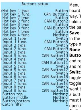
Menu items **Hot key 1** — **Hot key 4** — four buttons of the On-Button board computer, from left to right, are configured in the same way. The function assigned to them is activated by pressing and holding the button for 2 seconds. After setting, you need to save the parameters in the menu section **Onboard computer** > **Save.**
