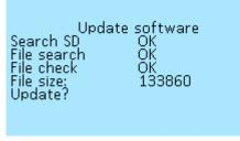
To update, download the firmware file to the root directory of the microSD card with Fat/Fat32 file system. Insert the card, with the contacts on top, into the connector on the On-board Computer. This can be done without turning off the On-board computer, but in this case, you must exit the **Update software** menu and reenter. After that, the On-board computer will detect the microSD card, display the **File size** in bytes and the menu item **Update**?
