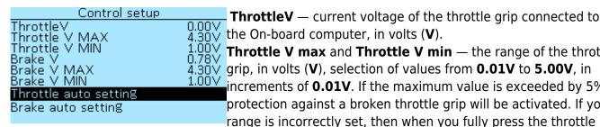
Throttle V max and Throttle V min — the range of the throttle grip, in volts (V), selection of values from 0.01V to 5.00V, in increments of **0.01V**. If the maximum value is exceeded by 5%, protection against a broken throttle grip will be activated. If your
