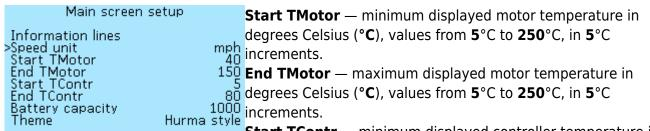
Start TContr — minimum displayed controller temperature in degrees Celsius (°C), values from 5°C to 250°C, in 5°C increments.
