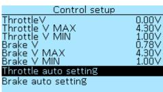
ThrottleV — current voltage of the throttle grip connected to 0.00 V the On-board computer, in volts (**V**).
