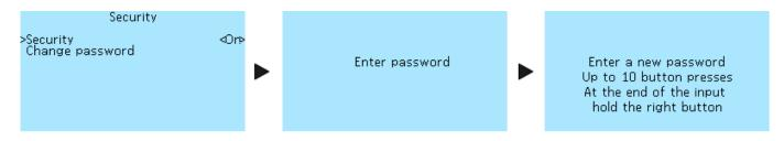
**Security** — enabling the password request function when starting the controller. Select **Off** and **On**.
