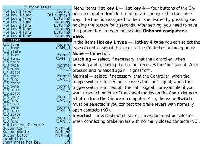
In menu items **Hot key 1 func.** — **Hot key 4 func.** selects the function assigned to the On-Board Computer button.
