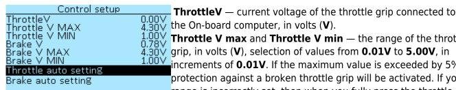
430 the On-board computer, in volts (**V**). Throttle V max and Throttle V min — the range of the throttle grip, in volts (V), selection of values from 0.01V to 5.00V, in increments of **0.01V**. If the maximum value is exceeded by 5%,
