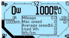
You can choose to display several types of statistics: **General**, **User**, **Trip**, **From charge**. For a detailed description, see the **Statistics** section. The main screen displays five parameters: **Mileage** — mileage in kilometers (**km**) or in miles (**mi**). **Max speed** — maximum speed, in kilometers per hour (**km/h**) or in miles per hour (**mph**).
