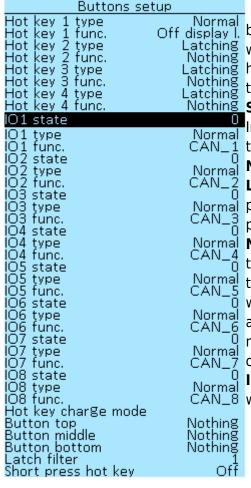
Menu items **Hot key 1** — **Hot key 4** — four buttons of the Onboard computer, from left to right, are configured in the same way. The function assigned to them is activated by pressing and holding the button for 2 seconds. After setting, you need to save the parameters in the menu section **Onboard computer** > **Save**.
