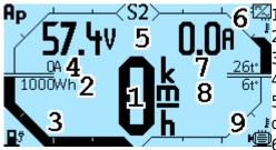
**6**<sup>[4]</sup>1. Speedometer or fast statistics, when the speed is zero.
