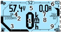
**6**<sup>[2]</sup>1. Speedometer or fast statistics, when the speed is zero.
