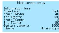
**Battery capacity** — the energy stored by the battery, in Watthours (W\*h), the values from **5** W\*h to **10000** W\*h, with increments of **5** W\*h.
