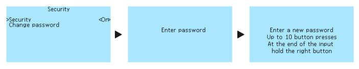
**Security** — enabling the password request function when starting the controller. Select **Off** and **On**. **Change password** — changing the default password.
