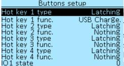
You can also configure the activation of charging by pressing and holding one of the buttons on the On-Board Computer (Hot key).
