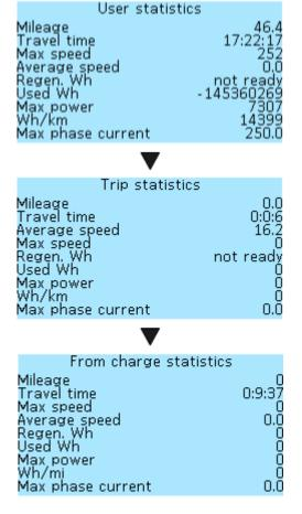
The list of parameters that are displayed for each type of statistics are the same and are calculated based on the type of statistics, with the exception of the **Charge Cycles** in the General statistics, instead of this item, in all other types of statistics is displayed the **Average speed** indicator, which is calculated while driving.
