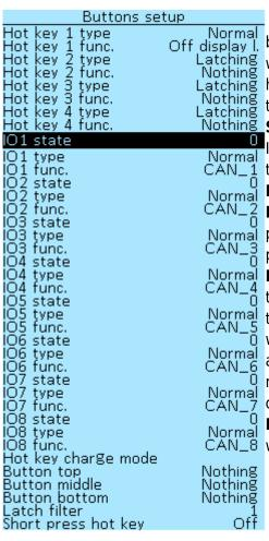
Menu items **Hot key 1** — **Hot key 4** — four buttons of the Onboard computer, from left to right, are configured in the same way. The function assigned to them is activated by pressing and holding the button for 2 seconds. After setting, you need to save the parameters in the menu section **Onboard computer** > **Save**.
