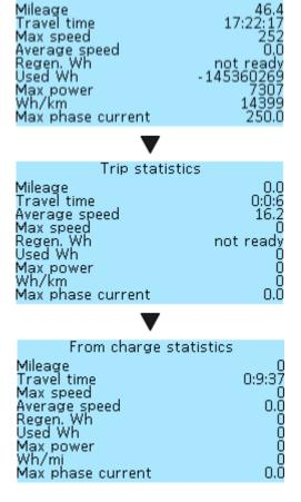
The list of parameters that are displayed for each type of statistics are the same and are calculated based on the type of statistics, with the exception of the **Charge Cycles** in the General statistics, instead of this item, in all other types of statistics is displayed the **Average speed** indicator, which is calculated while driving.
