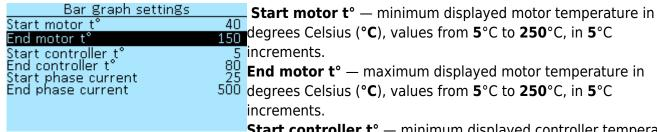
Start controller t° — minimum displayed controller temperature in degrees Celsius (°C), values from 5°C to 250°C, in 5°C increments.
