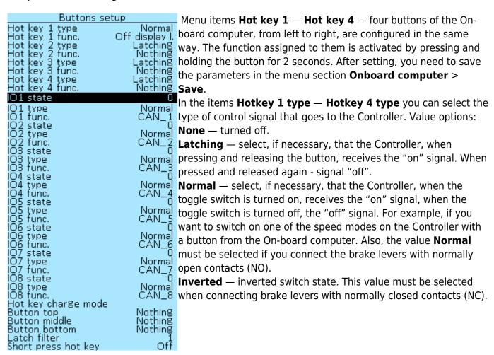
In menu items **Hot key 1 func.** — **Hot key 4 func.** selects the function assigned to the On-Board Computer button.
