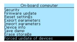
To update, download the firmware file to the root directory of the microSD card with Fat/Fat32 file system. Insert the card, with the contacts on top, into the connector on the On-board Computer. After that, go to the menu item **On-board computer > Forced update of devices** and select the device you want to update. Press the right button on On-board Computer to start the update. After restarting, check the firmware version under **On-board Computer > Device Information**.
