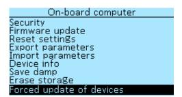
To update, download the firmware file to the root directory of the microSD card with Fat/Fat32 file system. Insert the card, with the contacts on top, into the connector on the On-board Computer. After that, go to the menu item **On-board computer > Forced update of devices** and select the device you want to update. Press the right button on On-board Computer to start the update. After restarting, check the firmware version under **On-board Computer > Device Information**.
