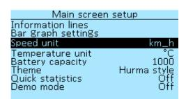
**Speed unit** — in kilometers per hour (**km\_h**) or in miles per hour (**mph**). **Temperature unit** — in degrees Celsius (°**C**) or degrees Fahrenheit (°**F**).
