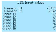
You can check the operation of the connected switch in the -37.7°C **Inputs values** menu section, when you turn the switch buttons  $^4_{
