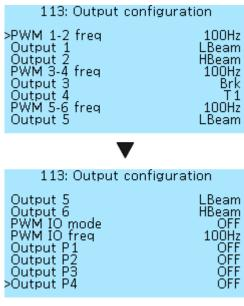
**PWM 1-2 freq** — a setting for advanced users. Selectable PWM 100Hz frequency values — 100Hz, 500Hz, 1kHz, 5kHz, 10kHz, 24kHz LBeam (FAN). For the usual light bulb, large values are not needed. <sup>100Hz</sup> Select a frequency of 100Hz, this will be enough not to see flicker.  $\frac{\text{Brk}}{\text{T1}}$  The high-frequency marked FAN is used to control the fans, this is 100Hz their standard frequency.
