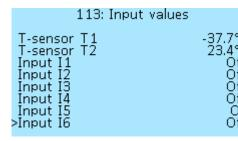
connected to **Input I5**, the second button will change the value of **Input I6**. Next, you need to configure the outputs and their functions in the menu of the uLight board. The order of settings does not matter, the main thing is that the output corresponds to the function and vice versa.
