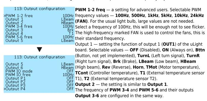
There is an **IO1** port on the uLight, in which there are four low-power PWM outputs **O1-O4**. They can connect, for example, an optocoupler. In the menu, you can select the mode of operation of the PWM at the outputs, its frequency, and the value of the function for each output. Outputs **O1** and **O2**, **O3** and **O4** can be connected in parallel to increase the total current.
