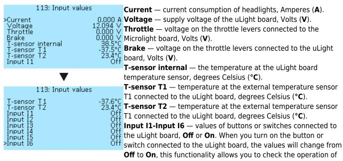
the buttons and to which board inputs they were connected.
