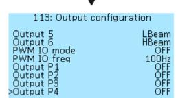
Output 1 — setting the function of output 1 (OUT1) of the uLight board. Selectable values — OFF (Disabled), ON (Always on), Bttn (Button, not yet implemented), TurnL (Left turn signal), TurnR (Right turn signal), Brk (Brake), LBeam (Low beam), HBeam (High beam), Rev (Reverse), Horn, TMot (Motor temperature), TCont (Controller temperature), T1 (External temperature sensor T1), T2 (External temperature sensor T2).
