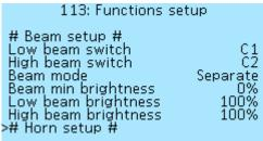
Next, select which button of the On-board computer the Low beam switch is connected to, we assigned the function **CAN**C1 Button1 to the first button, need to select the value C1. Next, we select which button of the On-board computer the High beam switch is connected to, we assigned the function **CAN Button2** to the second button, need to select the value **C2**. It is impossible to assign the inclusion of low and high beam to one button, only to
