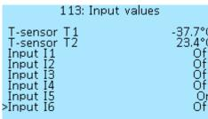
You can check the operation of the connected switch in the -37.7°C **Inputs values** menu section, when you turn the switch buttons 23.4°C off on and off, the value of one of the inputs **I1-I6** to which you off connected the switch will change from **Off** to **On**. You can also off use this menu to see what input number the connected switch  $rac{M}{2}$  has before the output configuration setup. In the example on the screenshot the left, we see that one of the switch buttons is
