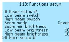
Next, select which button of the On-board computer the Low beam switch is connected to, we assigned the function **CAN Button1** to the first button, need to select the value **C1**. Next, we select which button of the On-board computer the High beam switch is connected to, we assigned the function **CAN Button2** to the second button, need to select the value **C2**. It is impossible to assign the inclusion of low and high beam to one button, only to
