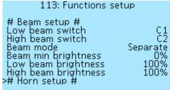
Next, select which button of the On-board computer the Low beam switch is connected to, we assigned the function **CAN**Separate select which button of the On-board computer the High beam switch is connected to, we assigned the function **CAN Button2** to the second button, need to select the value **C2**. It is impossible to assign the inclusion of low and high beam to one button, only to
