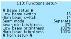
Next, select which output the low beam switch is connected to, for example, you connected a switch button to **Output 13**. Next, select which output the high beam switch is connected to, for example, to **Output 14**. It is impossible to assign the inclusion of low and high beam to one button, only to a switch or to two separate buttons. For a description of the **Single** and **Separate** beam modes, see above in the **Beam setup** menu section.
