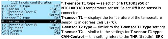
(brakes), **IO2**, and **IO3** inputs on the uLight board and is used when the throttle, brakes and switches are connected directly to the uLight board. When you select the **On** setting, control signals from the inputs will be transmitted via the CAN bus and you will be able to control the Controller from the uLight board using the throttle, brake and switch inputs.
